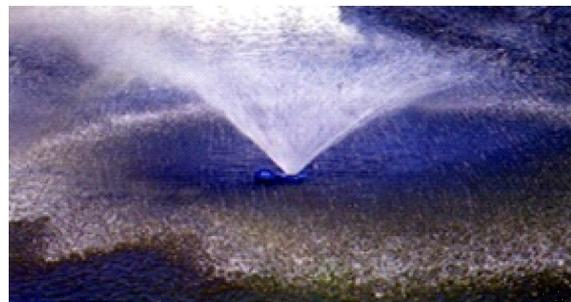
Figure 2: Pump-sprayer aerator
